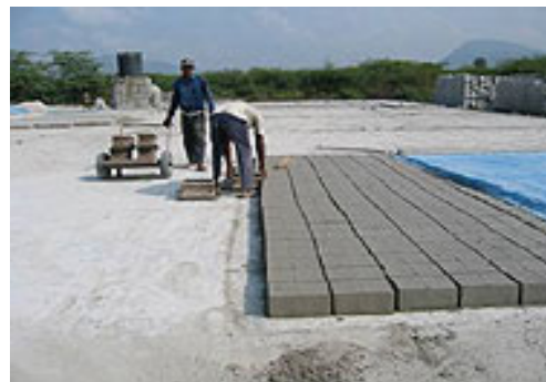
FaL-G bricks displaces coal for sintering
