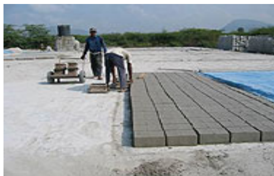
FaL-G bricks displaces coal for sintering
